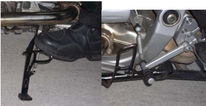
Left: An easy reach for retracting OR extending the side stand. Right: Modified loop of the RT stand neatly tucked against the bike does not interfere with shifting action.
